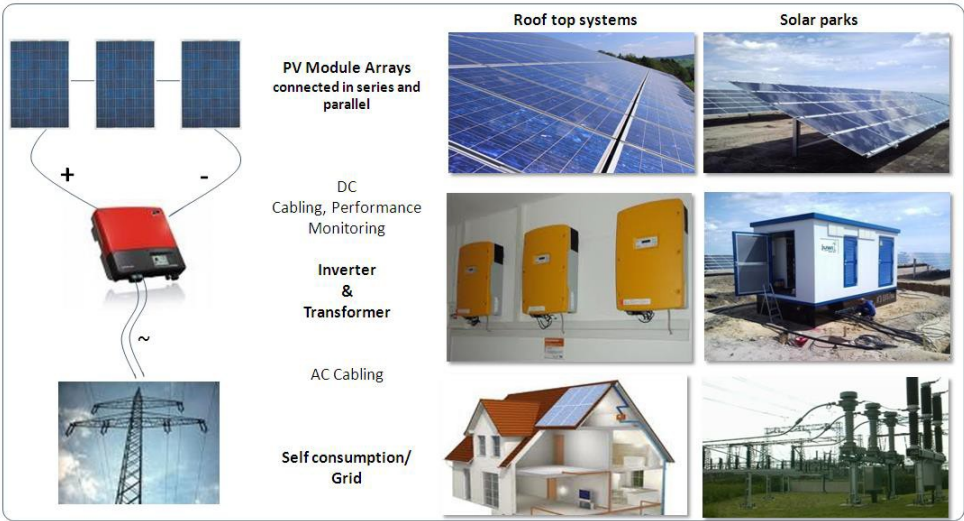
Fig. 11: PV system functional scheme
