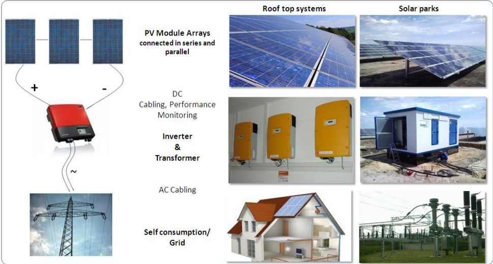
Fig. 11: PV system functional scheme
