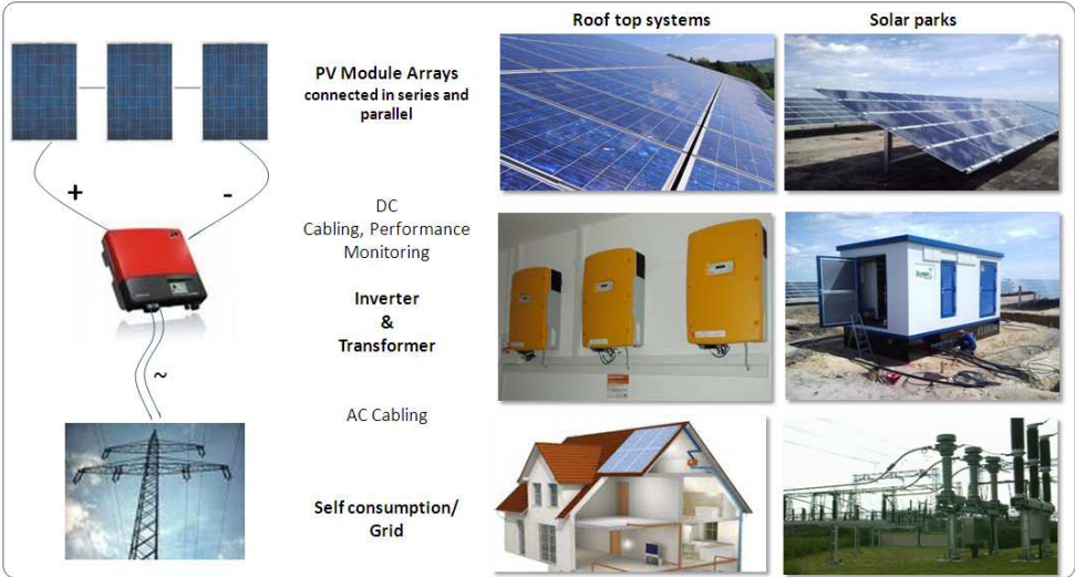
Fig. 12: PV system functional scheme
